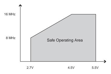
**Figure 159.** Maximum Frequency vs.  $V_{CC}$ , ATmega2560/ATmega2561
