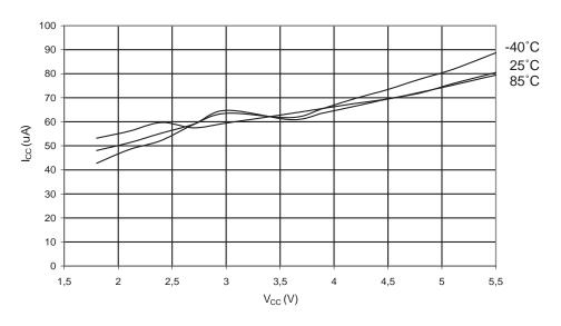
Figure 211. Programming Current vs. V<sub>CC</sub>
