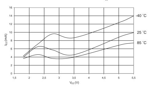
Current Consumption in Reset and Reset Pulsewidth
