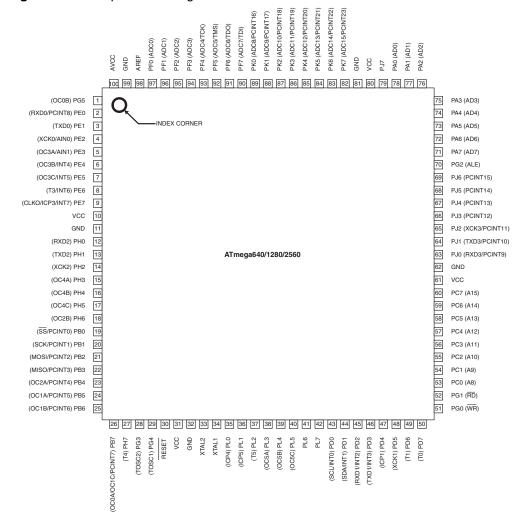
Figure 2. CBGA-pinout ATmega640/1280/2560
