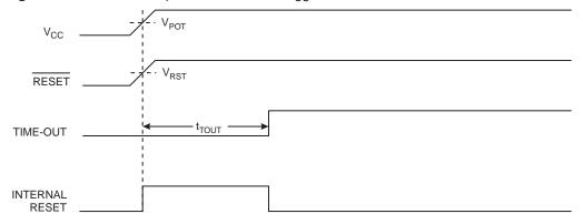
Figure 26. MCU Start-up, RESET Extended Externally
