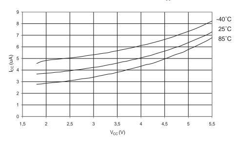
Figure 210. Analog Comparator Current vs. V<sub>CC</sub>
