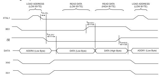
Note: 1. The timing requirements shown in Figure 144 (i.e., t<sub>DVXH</sub>, t<sub>XHXL</sub>, and t<sub>XLDX</sub>) also apply to reading operation.
