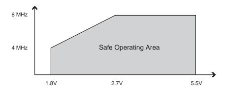
**Figure 157.** Maximum Frequency vs. V<sub>CC</sub> when only using No-Read-While-Write Section<sup>(1)</sup>, ATmega2560V/ATmega2561V
