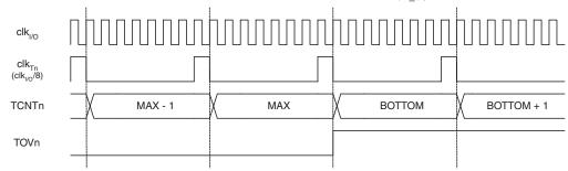
Figure 46 shows the setting of OCF0B in all modes and OCF0A in all modes except CTC mode and PWM mode, where OCR0A is TOP.
