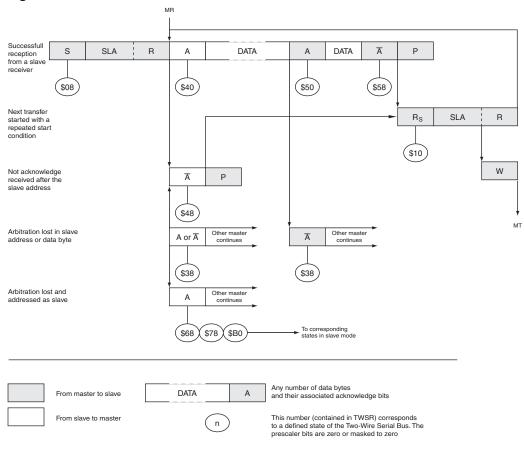
Figure 103. Formats and States in the Master Receiver Mode
