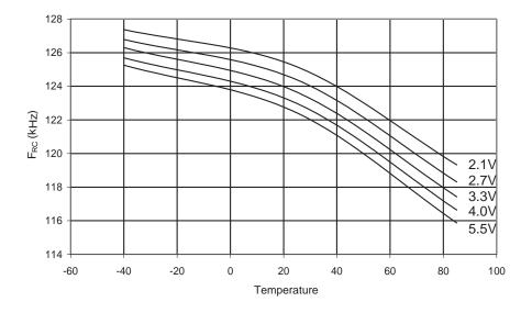
Figure 203. Calibrated 8 MHz RC Oscillator Frequency vs.  $\rm V_{CC}$  CALIBRATED 8 MHz RC OSCILLATOR FREQUENCY vs.  $\rm V_{CC}$
