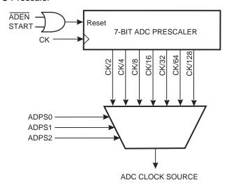
By default, the successive approximation circuitry requires an input clock frequency between 50 kHz and 200 kHz. If a lower resolution than 10 bits is needed, the input clock frequency to the ADC can be as high as 1000 kHz to get a higher sample rate.
