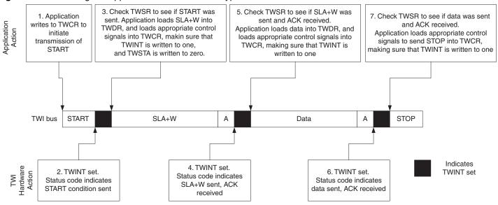
The first step in a TWI transmission is to transmit a START condition. This is
