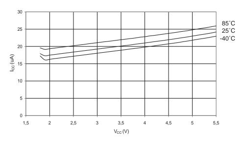
Figure 207. ADC Current vs.  $V_{CC}$  (AREF =  $AV_{CC}$ )
