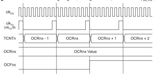
Figure 59 shows the count sequence close to TOP in various modes. When using phase and frequency correct PWM mode the OCRnx Register is updated at BOTTOM. The timing diagrams will be the same, but TOP should be replaced by BOTTOM, TOP-1 by
