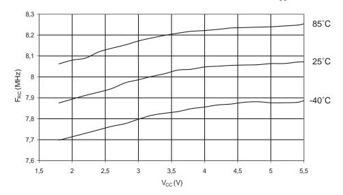
Figure 204. Calibrated 8 MHz RC Oscillator Frequency vs. Temperature
