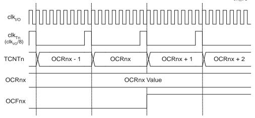
Figure 76 shows the setting of OCF2A and the clearing of TCNT2 in CTC mode.
