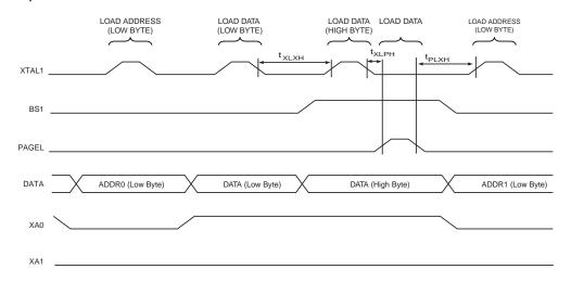
Note: 1. The timing requirements shown in Figure 144 (i.e., t<sub>DVXH</sub>, t<sub>XHXL</sub>, and t<sub>XLDX</sub>) also apply to loading operation.
