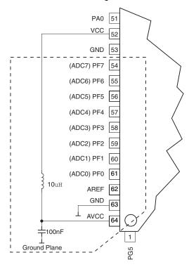
Figure 122. ADC Power Connections, ATmega640/1280/2560
