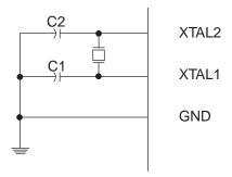
The Low Power Oscillator can operate in three different modes, each optimized for a specific frequency range. The operating mode is selected by the fuses CKSEL3:1 as shown in Table 12.
