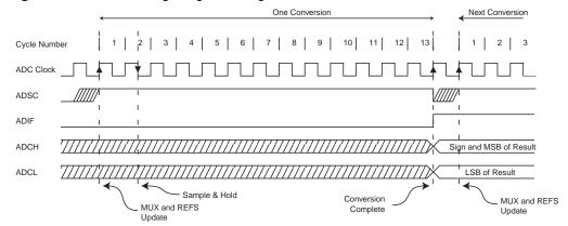
Figure 118. ADC Timing Diagram, Auto Triggered Conversion
