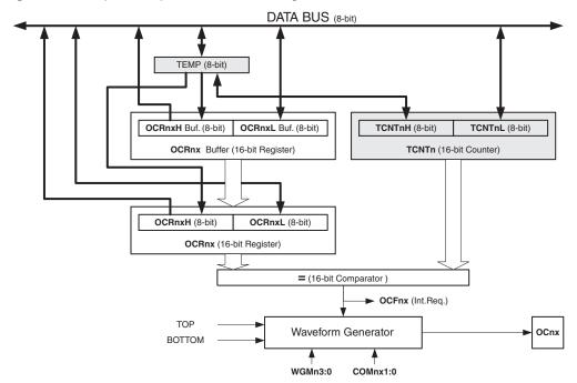
Figure 51. Output Compare Unit, Block Diagram
