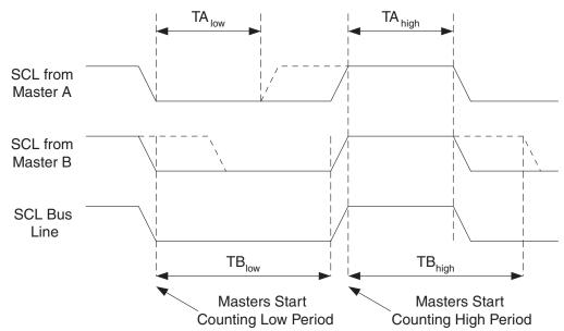
Figure 96. SCL Synchronization Between Multiple Masters
