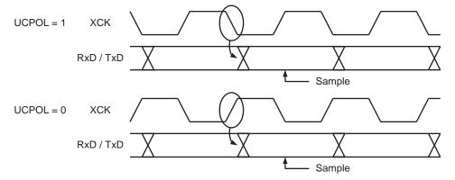
The UCPOLn bit UCRSC selects which XCKn clock edge is used for data sampling and which is used for data change. As Figure 84 shows, when UCPOLn is zero the data will be changed at rising XCKn edge and sampled at falling XCKn edge. If UCPOLn is set, the data will be changed at falling XCKn edge and sampled at rising XCKn edge.
