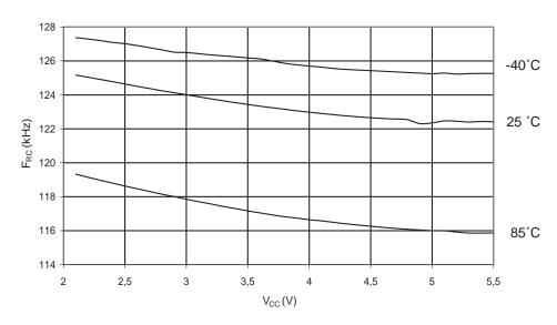
Figure 202. Watchdog Oscillator Frequency vs. Temperature
