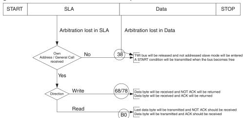
Figure 110. Possible Status Codes Caused by Arbitration
