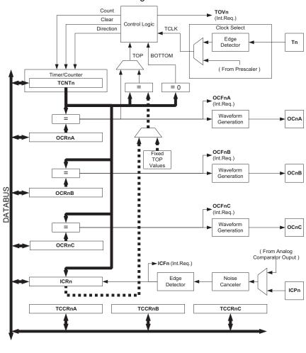
Figure 48. 16-bit Timer/Counter Block Diagram<sup>(1)</sup>
