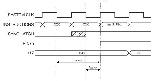
Figure 34. Synchronization when Reading an Externally Applied Pin value
