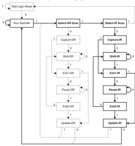
Figure 150. State Machine Sequence for Changing the Instruction Word
