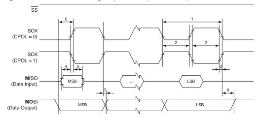
Figure 162. SPI Interface Timing Requirements (Slave Mode)
