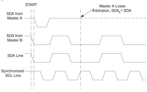
Figure 97. Arbitration Between Two Masters
