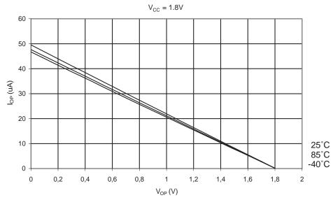
I/O PIN PULL-UP RESISTOR CURRENT vs. INPUT VOLTAGE
