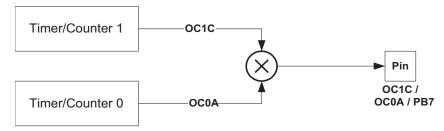
When the modulator is enabled, the two output compare channels are modulated together as shown in the block diagram (Figure 63).
