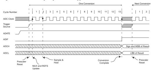
Figure 119. ADC Timing Diagram, Free Running Conversion
